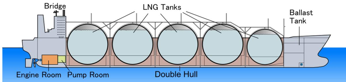
Moss-style LNG tankers use individual, spherical storage tanks built separately and set in place in the hull.
